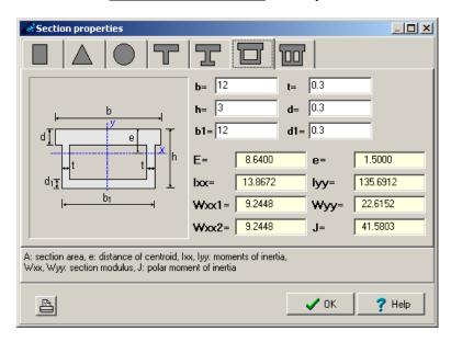
So we have Iyy=135.7 ft4, Ixx=13.9 ft4, A =8.64 ft2, J=41.58 ft4, Io=Ixx+Iyy=149.60 ft4 Mass (underwater part) mx = my = 12x2.5x0.064/32.2 =0.06 k slug/ft, mt=149.60x0.06/8.64=1.03 k slug ft2/ft (0.064 water specific weight, 32.2 acceleration of gravity)
